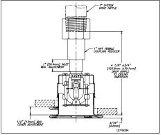
Fig. 3 - 1" NPT Female-Adjustable Inlet
