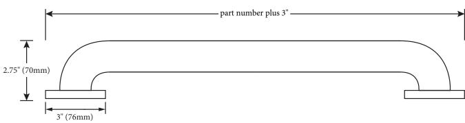
Holes - 0.25" (6mm) Slots - 0.25" (6mm) x 0.5" (13mm) (used when installing with the WINGITS® Grab Bar Fastening System)
