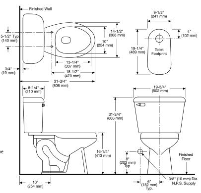
NOTE: Install this product according to the installation guide. Fixture dimensions are nominal and conform to tolerances in ASME Standard A112.19.2
