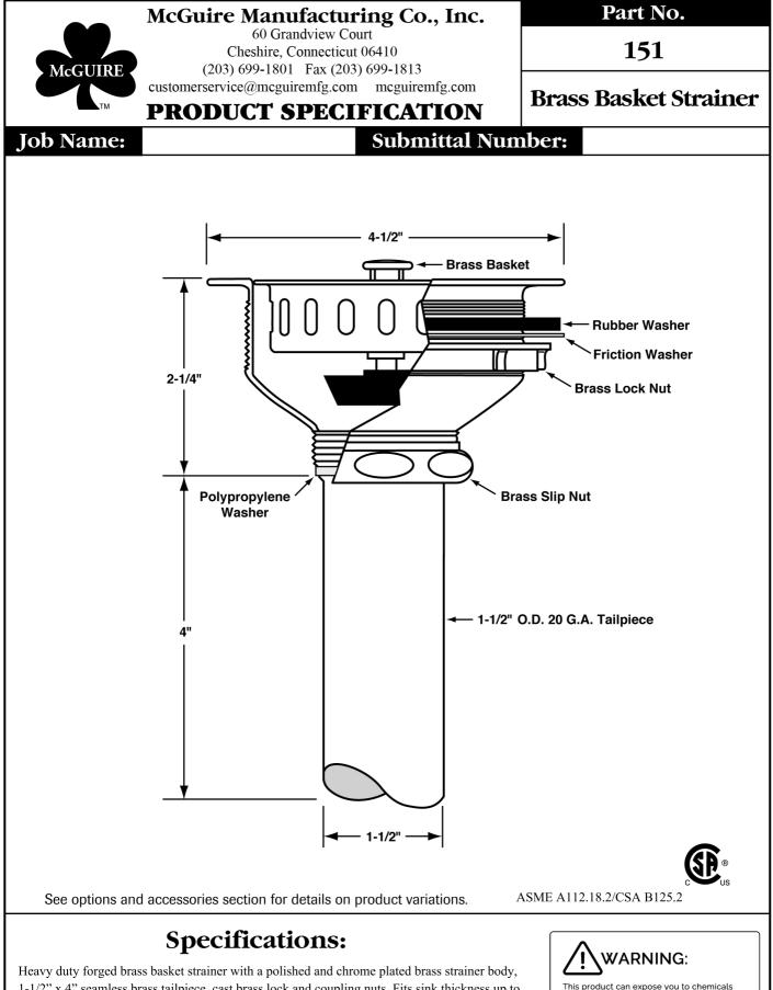
Heavy duty forged brass basket strainer with a polished and chrome plated brass strainer body, 1-1/2" x 4" seamless brass tailpiece, cast brass lock and coupling nuts. Fits sink thickness up to 5/8". Basket strainer in compliance with CSA or other recognized testing authority and bear both manufacturer and testing mark.
