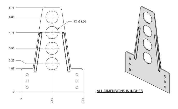
The LOCKRITE<sup>TM</sup> #609-N-6 is a 16 gage galvanized steel bracket with 1" holes on 1-1/4" centers. Ideal for toilets or hose bib stub-outs. Also serves as a nail plate. This bracket is designed to work exclusively with our glueable HOLDRITE<sup>®</sup> #604 ( $\frac{1}{2}$ ") or #605 ( $\frac{3}{4}$ ") inserts when installing CPVC tubing. Inserts snap into bracket.
