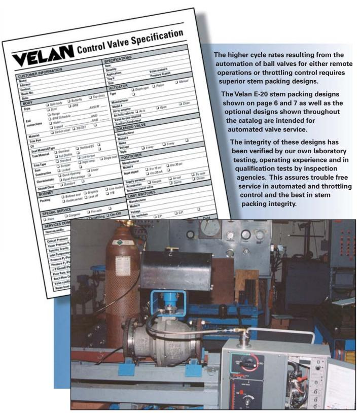
TA-LUFT qualification test on a 6" (150 mm) SB-150 ball valve.
