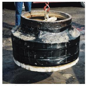
WrapidSeal™ adhesive strength demonstrated with vertical lift.
