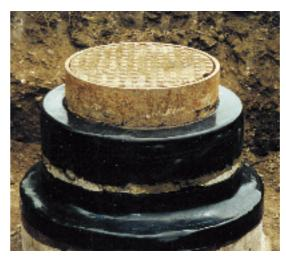
High expansion backing conforms and recovers to irregular structures.
