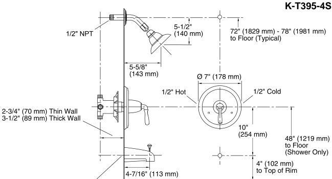
For slip-fit spout, 5/8" OD tube must extend 3-1/4" (83 mm) max beyond the finished wall.
