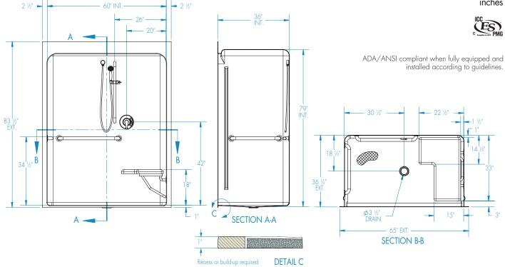
FEATURES Dimensional Tolerance ± %". Dimensions needed for site preparation should be measured from the unit. Aquatic assumes no responsibility for preparatory work.
