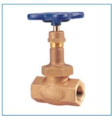
**Specifications UPC** Code 039923629586 Type Globe Valve **Valve Size** 1/2 T -- Female NPT Thread (FIPT) **Connection Type** Material **Bronze** Standard Handwheel **Valve Operator** T275Y 1/2 THD 300# GLOBE PTFE SEAT **Description** eClass Classification Bronze Globe Valves **Turns/Operation** Multi-Turn Weight 1.823 lb
