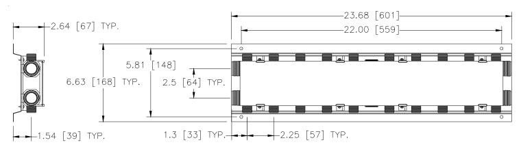
Engineering Specification: ZumPEX® 1"diameter polysulfone QickPort® Pre-Assembled Manifold comprised of ten (10) hot and ten (10) cold 1/2" male straight pipe thread outlets and four (4) 1" male pipe straight thread inlets. Manifold is rated at a maximum pressure of 100 PSI at 180°F. Optional shut off valves can be added for individual on/off control of each distribution line. NSF listed. For use with potable water only.
