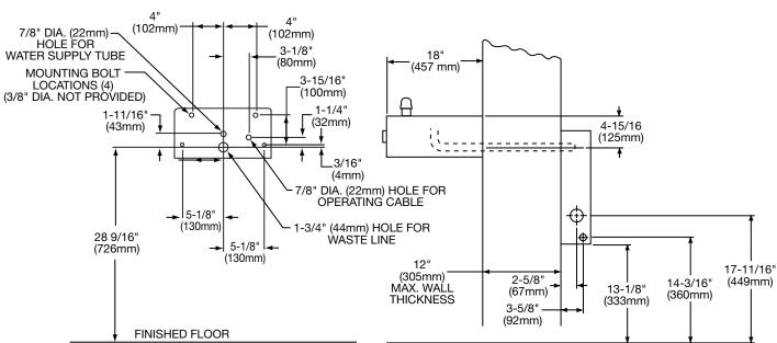
NOTE: ALL DIMENSIONS ARE TAKEN FROM THE FINISHED FLOOR ON THE SIDE OF THE WALL THAT THE FOUNTAIN IS ON.
