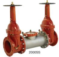
Series 2000SS Double Check Valve Assemblies are designed to prevent the reverse flow of polluted water from entering into the potable water system. This series can be applied, where approved by the local authority having jurisdiction, on non-health hazard installations. Features short end-to-end dimensions, lightweight stainless steel body, and low head loss.
