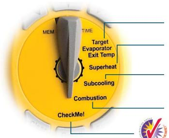
Determine actual and **target evaporator exit temperature** by taking three temperature measurements.
