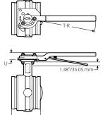
VALVE WITH LEVER LOCK HANDLE AND MEMORY STOP 8"/200 MM SIZES
