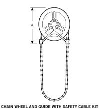
Chain wheels are mounted to the gear operator handwheels. Sprocket rim and guide arms are made of cast aluminum. Chain is galvanized steel.
