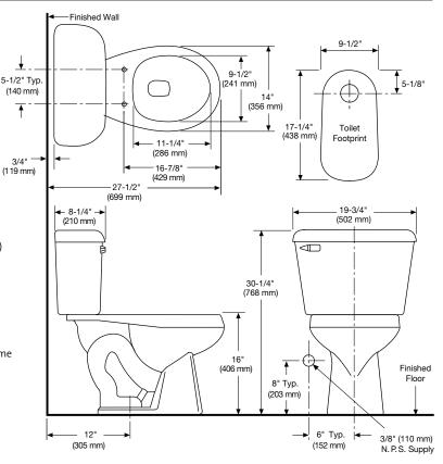
NOTE: Install this product according to the installation guide. Fixture dimensions are nominal and conform to tolerances in ASME Standard A112.19.2
