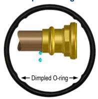
The Drip Fit o-rings (up to 2") ensure that an unpressed end will drip. This is an added safety feature to ensure unpressed ends are discovered and corrected.
