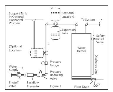
Install the expansion tank in the incoming water line to the water heater between the water heater and the backflow preventer or check valve (see Fig. 1). Adequate thread sealant must be added to ensure a leak-free installation.
