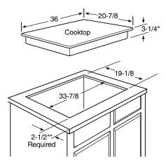
\*Depth of unit at conduit connection location (rear) is 6-1/4" on models PP980/975/950/945 and 4-5/8" on models PHP960/900, PP972/962/942/932/912 and JP6SS/356/346/340.
