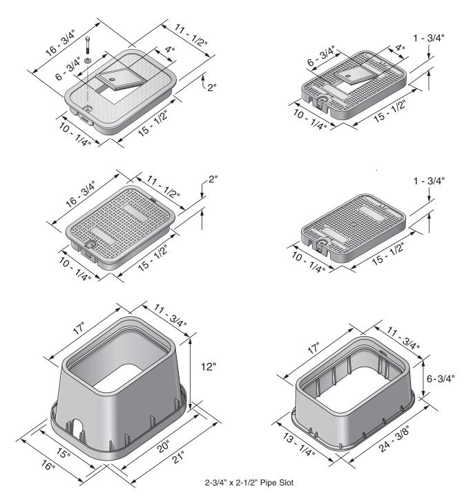
Product is not to be installed in concrete and is not to be used in vehicular applications. Weights and dimensions are nominal.
