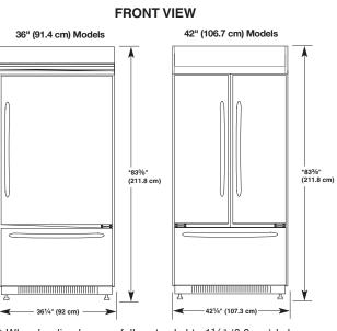
\* When leveling legs are fully extended to 11/4" (3.2 cm) below rollers, add 1<sup>1</sup>/<sub>8</sub>" (2.9 cm) to the height dimensions.
