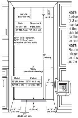
A clearance of 1/2" (1.3 cm) must be maintained in front of the refrigerator's side trim in order for the top grille to be removed.
