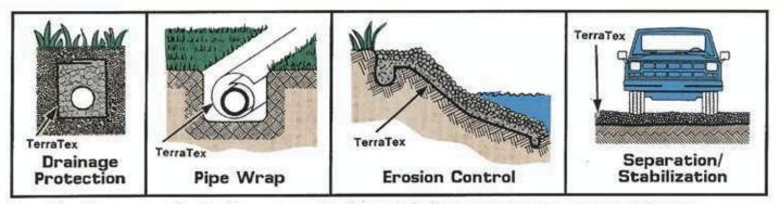
TerraTex Nonwoven Geotextiles are made of specially formulated polypropylene to insure resistance to most soil chemicals, rot, mildew, acids, and alkalies in a pH range from 3 to 12.
