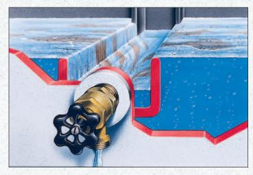
Built-in speed skimmer trough dramatically reduces steam boiler cleaning time.
