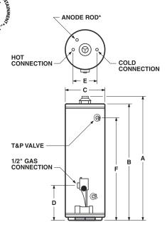
\*Location for optional top-mounted T&P Valve, if ordered from factory (C3 models only). To order, add "G" to model number (GSX 40 YRRT **G**).
