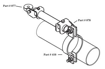
SIZE - SYSTEM PIPE: Nominal Pipe Size Sch. 40 Steel 1" thru 8" Sch. 10 Steel 1 1/4" thru 8" MATERIAL - Carbon Steel FINISH - Plain or E.G. LISTING/APPROVAL -
