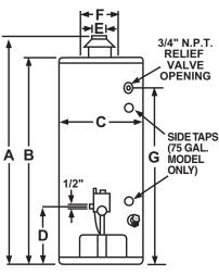
G60-50 & G75-75 SIDE TAPS ON 75 GAL. MODEL ONLY G60-50 WATER CONNECTIONS ARE 3/4" NPT G75-75 WATER CONNECTIONS ARE 1" NPT
