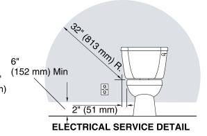
The receptacle should be located at least 6" (152 mm) above the floor line, and within a 32" (813 mm) radius measured 2" (51 mm) to the right of the toilet ledge, as shown.
