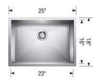
Undermount installation only Minimum cabinet size: 30'' Cut-out Dimensions: Cut-out Length: 23.24'' Cut-out Width: 16.24'' Cut-out Below Counter Depth: 10.79'' Sink Bowl Dimensions: Sink Bowl Length (left-to-right): 23'' Sink Bowl Length (left-to-right): 23'' Sink Bowl Width (front-to-back): 16'' Sink Bowl Depth: 10'' Drain hole compatible with 3.5'' strainers or waste flanges Codes/Standards: ASME A112.19.3-2017/CSA B45.4-17
