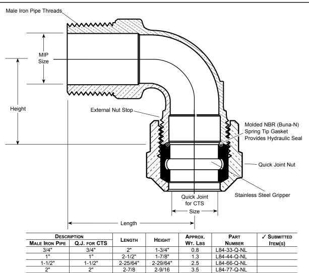
Note: Ford recommends insert stiffeners when using plastic pipe or tubing.
