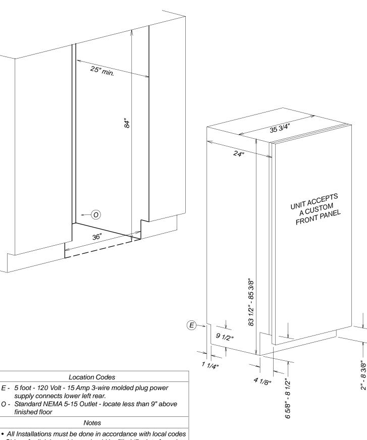
• Sides of adjoining cabinets should be filled (flush to frame) to insure proper fit and finish
