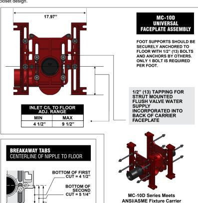
**Note:** 8" tapered thread ABS nipple shipped standard with MC-10 Series carriers. The universal assembly accepts all nipple variations, rolling thread (-OR), cast iron (-CI) and tapered thread ABS with adjustable horn (-AH).
