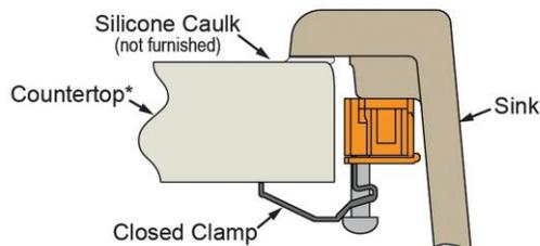
\*Maximum thickness for use of hold down system is 1-3/4" (44mm).
