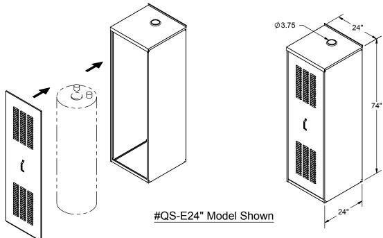
The HOLDRITE® QUICK SHED™ Water Heater Enclosures are constructed of galvanized steel and provide protection for water heaters installed in outdoor locations. Anchor points at the rear of the enclosure allows for optional attachment to the adjacent building structure.
