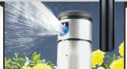
I-20-12: Overall height: 17" Pop-up height: 12" Exposed diameter: 1¾" Inlet size: ¾" female NPT
