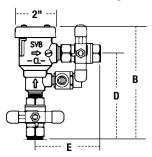
A strainer is recommended to be installed ahead of the backflow preventer to prevent the fouling of the check assembly and resulting spillage from the valve during repressurization. Do not install in concealed locations or areas where water leakage due to normal wear of the internal parts can cause damage.
