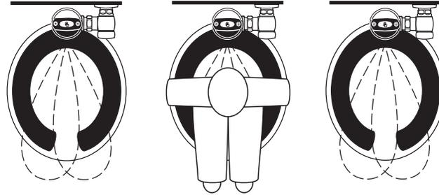
1. A continuous, invisible light beam is emitted from the OPTIMA Plus® Sensor.
