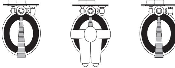
1. A continuous, invisible light beam is emitted from the OPTIMA® Sensor.
