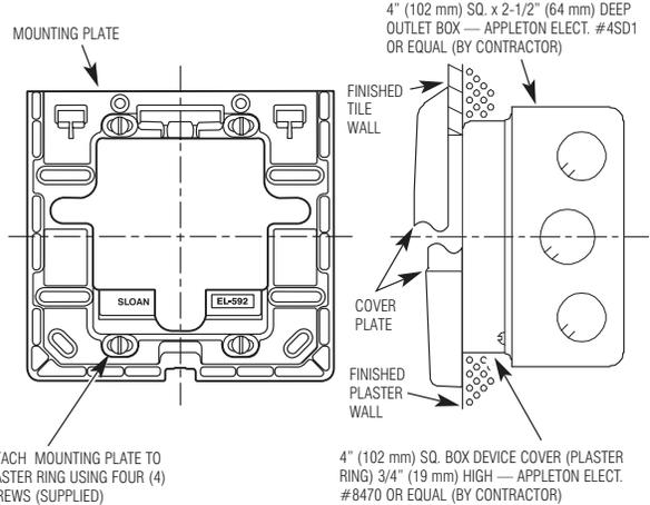
ATTACH MOUNTING PLATE TO PLASTER RING USING FOUR (4) SCREWS (SUPPLIED)
