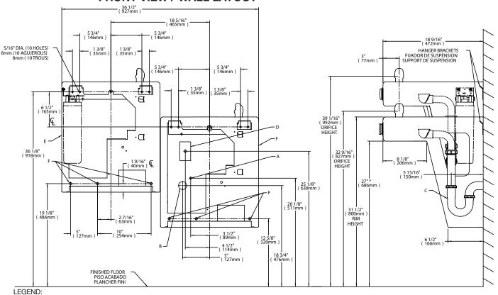
A = RECOMMENDED WATER SUPPLY LOCATION. SHUT OFF VALVE (NOT FURNISHED) TO ACCEPT 3/8" O.D. UNPLATED COPPER TUBE.
