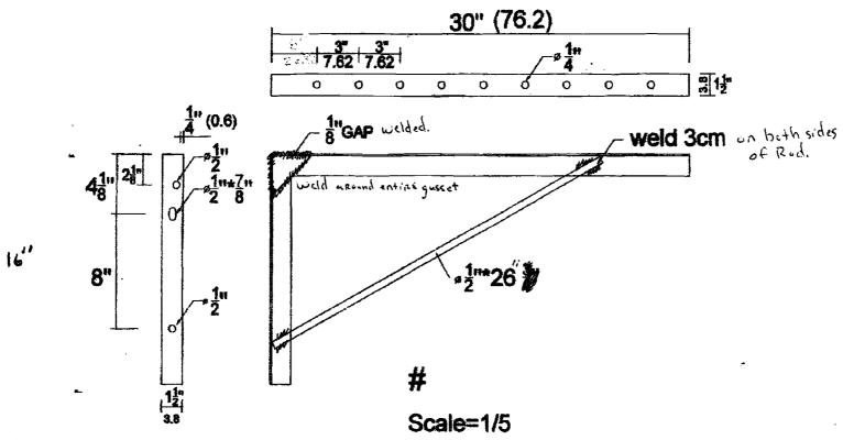
Angle iron size 3.8Cm\*3.8Cm Material Steel 2.8mm Finished Grey Power Coating 3.0mm
