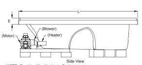
Н Overall Height\*\* 24" 610 mm Overflow Height 17" 432 mm Α 10 1/4" B Long Edge to Drain Center 260 mm С Short Edge to Drain Center 17 11/16" 447 mm 7" D Drain Shoe Length 178 mm 4" Ε Deck Height\*\* 102 mm Deck Width\* 76 mm G Service Access Dimensions 12" H x 18" L 305 mm x 457 mm 12" x 4" 305 mm x 102 mm Floor Cut-out for Drain
