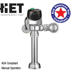
Sloan ECOS® Hardwire Dual Flush Flushometers incorporate intuitive split-button design for easy manual activation. The small green button controls the reduced flush cycle (1.1 gpf/4.2 Lpf), the large button controls the full flush cycle (1.6 gpf/6.0 Lpf). Straightforward graphics alert user to proper activation. Reduced flush for liquid waste, full flush for solid waste. To further educate the user, two (2) instructional wall plates are included with each Sloan ECOS® Flushometer.
