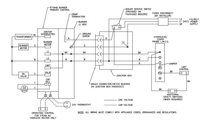
Figure 4.4: Steam with Probe Low Water Cut-Off
