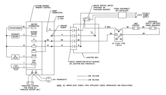
Figure 4.3: Steam with Float Low Water Cut-Off
