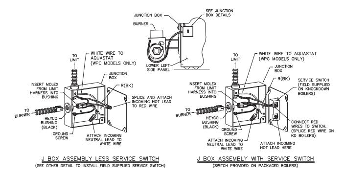
Figure 4.1: Junction Box Wiring
