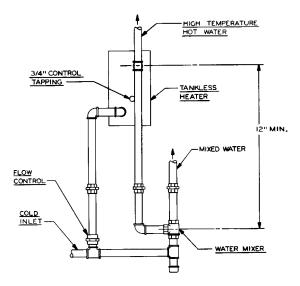
Figure 3.3: Tankless Coil Piping, Steam Boiler
