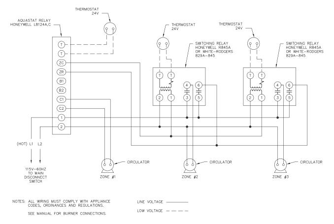
Figure 4.6: Zoning with Circulators, Honeywell L8124A, C Aquastat
