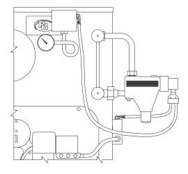
Figure 3.7: Float Low Water Cut-off
