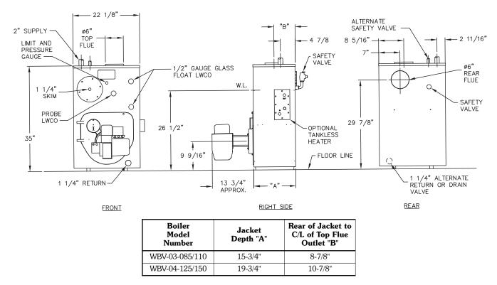
Figure 7.2: Boiler Dimensions, Steam Boiler
