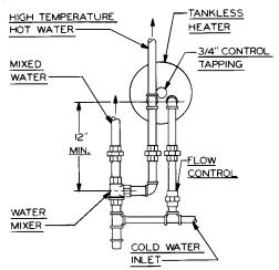
Figure 3.4: Tankless Coil Piping, Water Boiler
