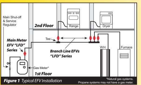
AutoTrip Meter (LFD) Excess Flow Valves are designed to be positioned after (downstream from) the gas meter. In this location, the valve is designed to protect against a catastrophic failure of the main trunk line. In order to protect the smaller downstream branch lines, the smaller LFD branch line valves (-70 and -125) may be positioned within a branch line serving one or more appliances. Excess Flow Valves are gravity dependent and must be installed in the vertical
