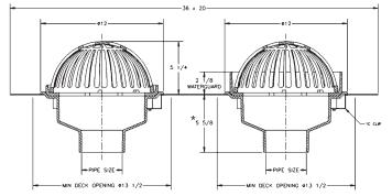
\* 5-5/8" DIM. (BODY HGT.) VARIES BY OUTLET SIZE WITH -T AND -X CONNECTIONS.
