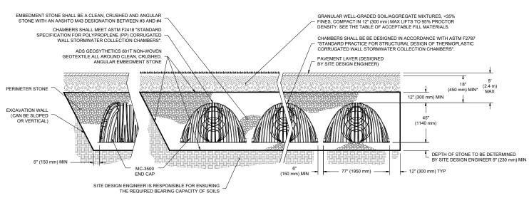
\*MINIMUM COVER TO BOTTOM OF FLEXIBLE PAVEMENT. FOR UNPAVED INSTALLATIONS WHERE RUTTING FROM VEHICLES MAY OCCUR, INCREASE COVER TO 24" (600 mm)
