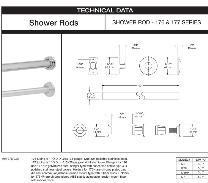
INSTALLATION: Install hanger type flanges and rod with 4 - #8 X 1-1/4" round head zinc plated steel screws provided. Cover flanges to be on rod before installation of hangers and rod. Slide cover flanges over hangers to complete installation. Install adjustable tension mounted holders and rod by sizing rod 1-5/8" shorter than wall opening. Insert rod into holders and tighten into position with counterclockwise motion on threaded holder until secure.
