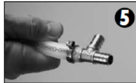
Verify connection is secure. Use go/no-go gauge on crimp rings.
