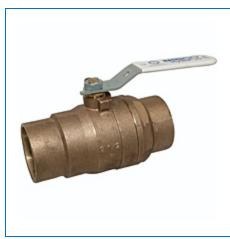
**Specifications UPC** Code 039923338938 Ball Valve Type Valve Size 2 1/2 in **Body Material** Lead Free Silicon Bronze **Seat Material** RPTFE (Reinforced) **Seal Material** RPTFE (Reinforced) Stem Material Stainless Steel ASTM A276 Type 316 CS Standard Lever Handle **Operation Type Connection Type** S -- Female Solder Cup **Ball Material** Stainless Steel
