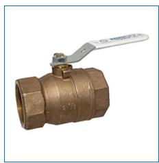
**Specifications UPC** Code 039923339034 Ball Valve Type Valve Size 2 1/2 in **Body Material** Lead Free Silicon Bronze **Seat Material** RPTFE (Reinforced) **Seal Material** RPTFE (Reinforced) Stem Material Stainless Steel ASTM A276 Type 316 CS Standard Lever Handle **Operation Type** T -- Female NPT Thread (FIPT) **Connection Type Ball Material** Stainless Steel
