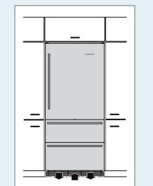
CS 20 appliances dont need any ventilation openings in the cabinet. The required airflow is directed through the toe kick area.
